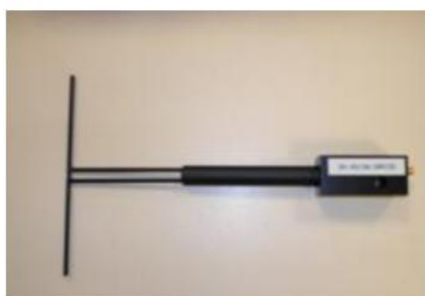
Figure 1 – Satimo COMOSAR Validation Dipole
