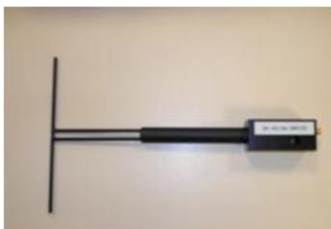
Figure 1 – Satimo COMOSAR Validation Dipole
