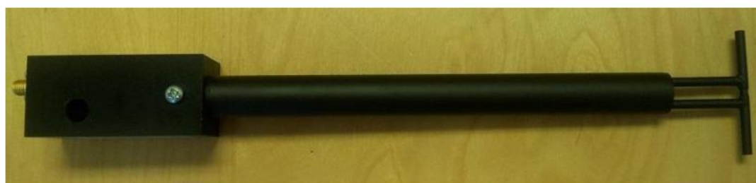
Figure 1 – MVG COMOSAR Validation Dipole
