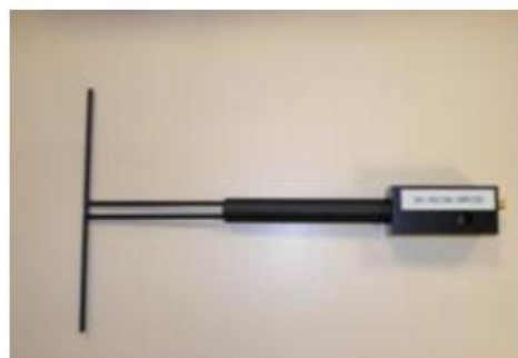
Figure 1 – Satimo COMOSAR Validation Dipole
