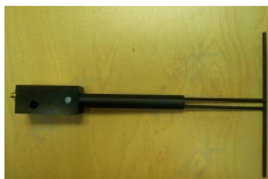
Figure 1 – MVG COMOSAR Validation Dipole
