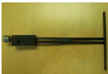
Figure 1 – MVG COMOSAR Validation Dipole
