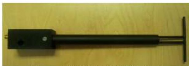
Figure 1 – MVG COMOSAR Validation Dipole
