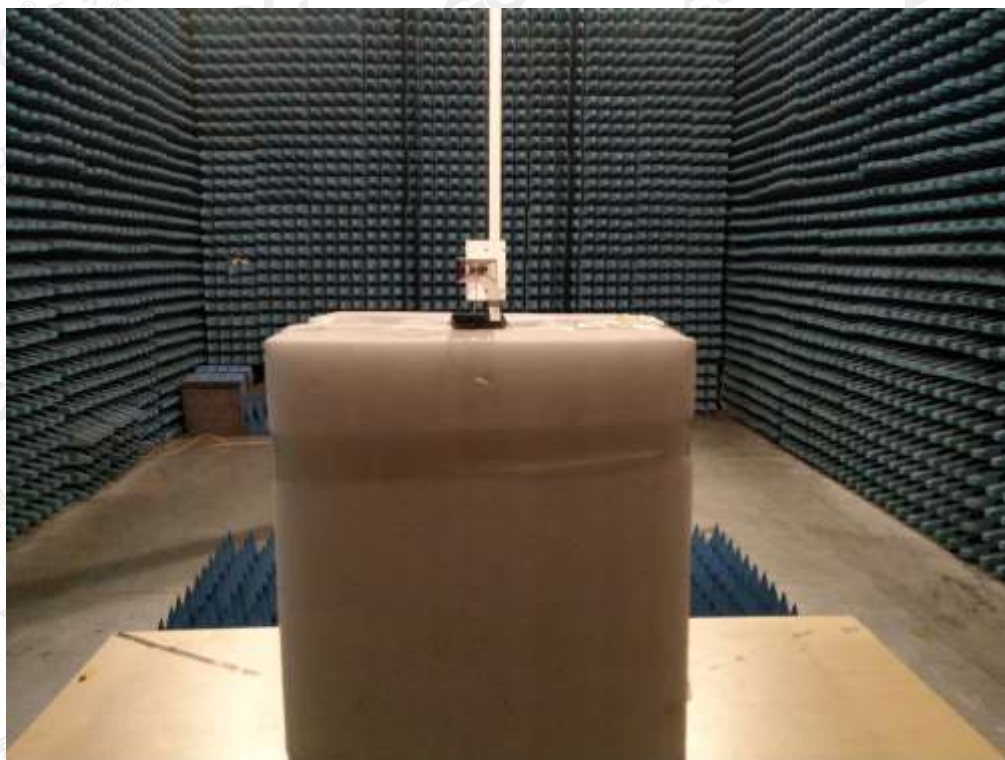
RADIATED SPURIOUS EMISSION-ABOVE 1G TEST SETUP
