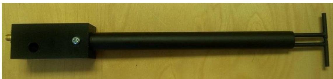
Figure 1 – MVG COMOSAR Validation Dipole
