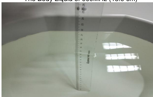
The Body Liquid of 2000MHz (16.5cm)
