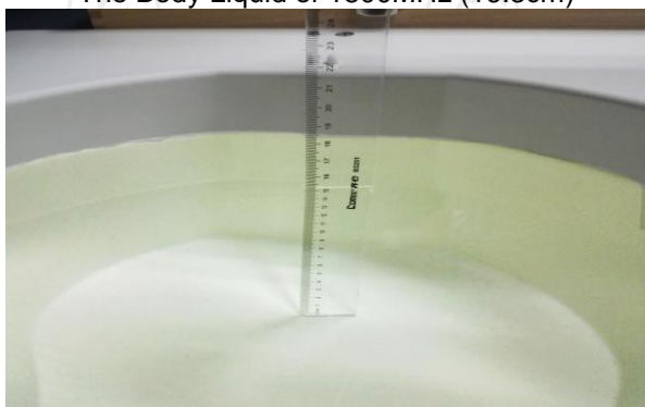
The Body Liquid of 5000-6000MHz (15.2 cm)
