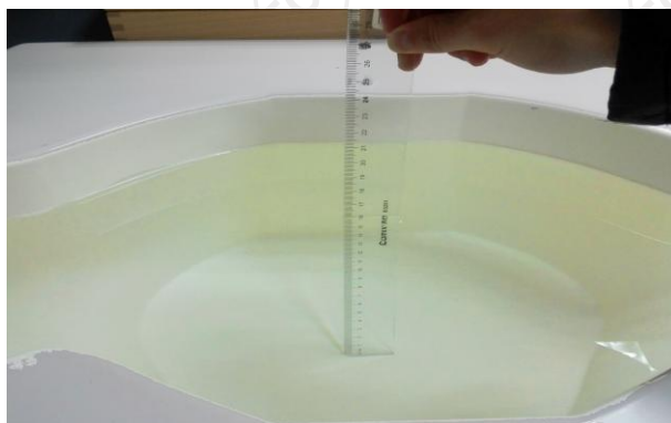
The Body Liquid of 900MHz (15.9 cm)
