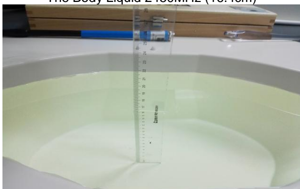
The Body Liquid of 1800MHz (16.3cm)
