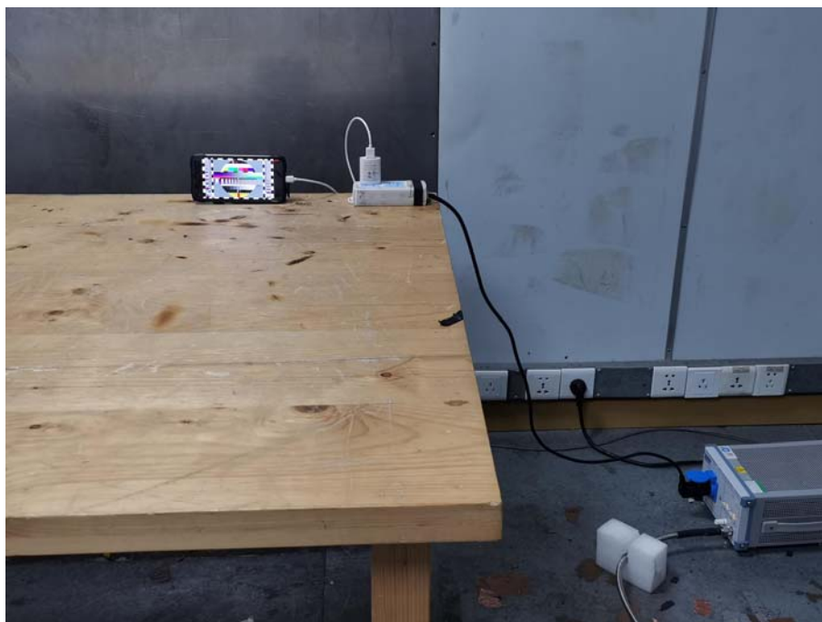
Photo of Conducted Emission Measurement
