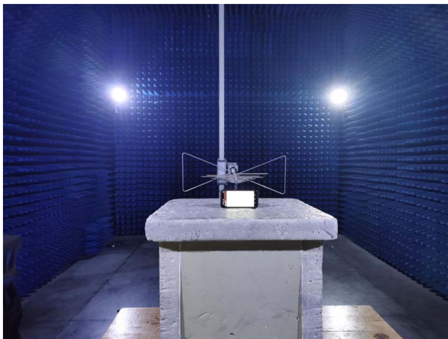
Photo of Radiated Emission Measurement (Below 1G)
