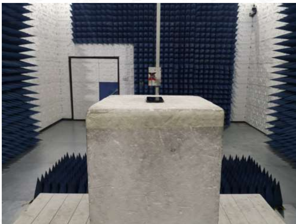
RADIATED SPURIOUS EMISSION-ABOVE 1G TEST SETUP
