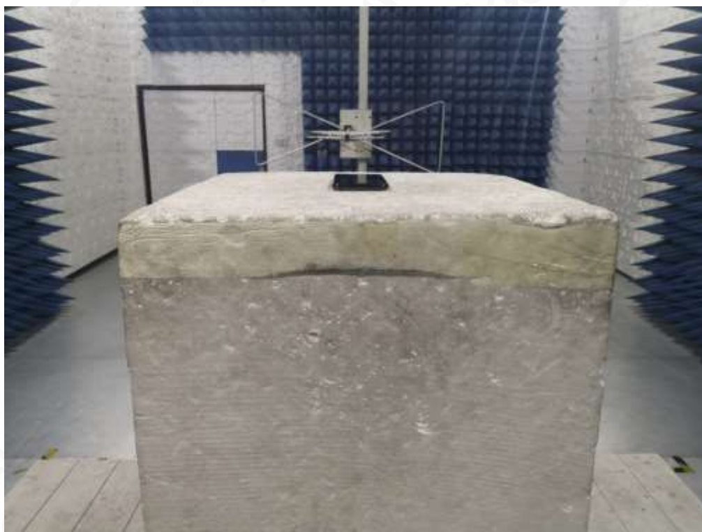
RADIATED SPURIOUS EMISSION-ABOVE 1G TEST SETUP
