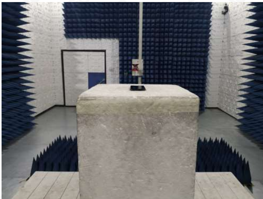
RADIATED SPURIOUS EMISSION-ABOVE 1G TEST SETUP
