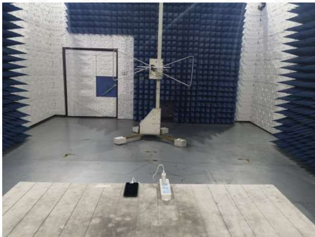
EN 55032 RADIATED EMISSION TEST SETUP
