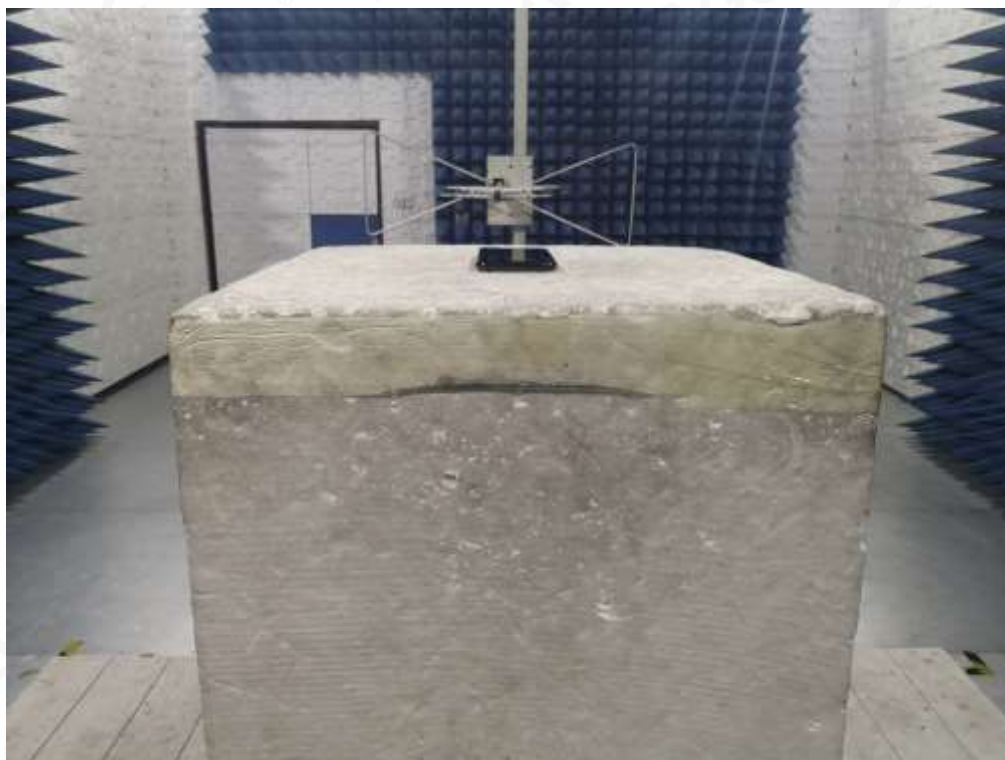
RADIATED SPURIOUS EMISSION-ABOVE 1G TEST SETUP
