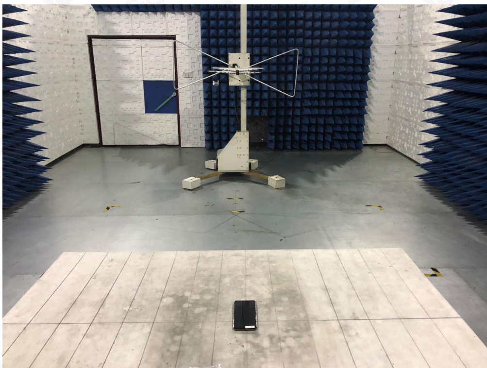
RADIATED EMISSION TEST SETUP
