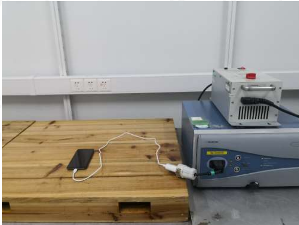
EFT SURGE and DIPS IMMUNITY TEST SETUP
