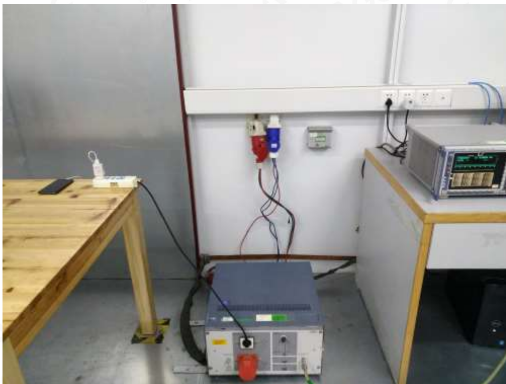
EN 55032 RADIATED EMISSION TEST SETUP
