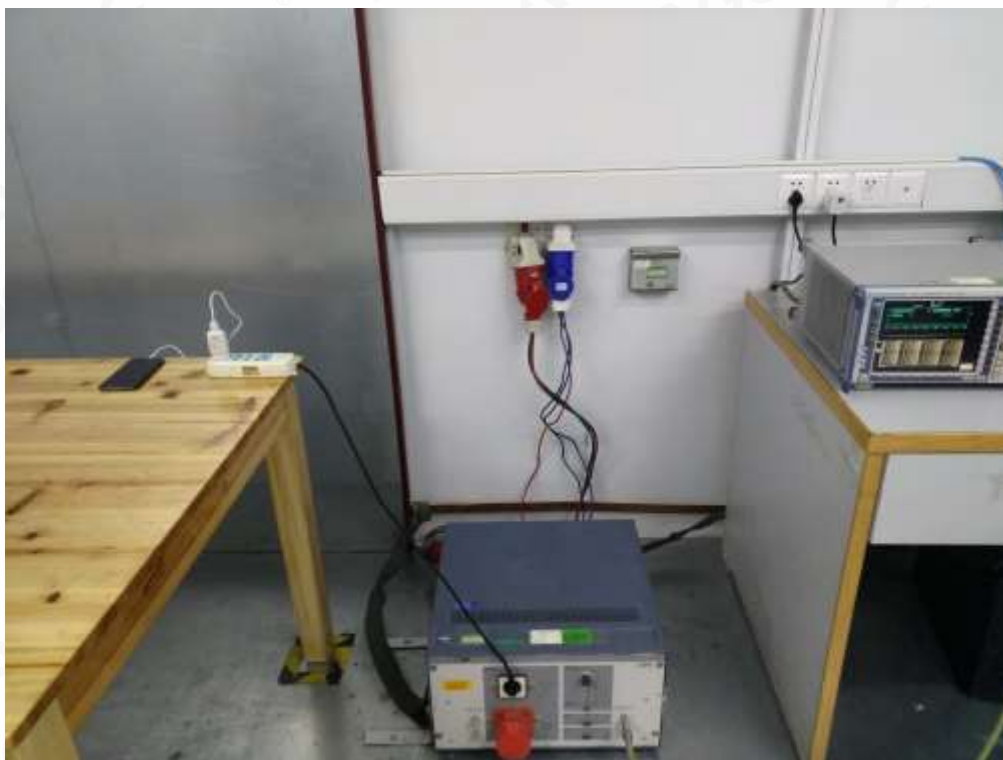
EN 55032 RADIATED EMISSION TEST SETUP
