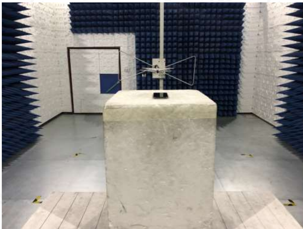
RADIATED SPURIOUS EMISSION-ABOVE 1G TEST SETUP
