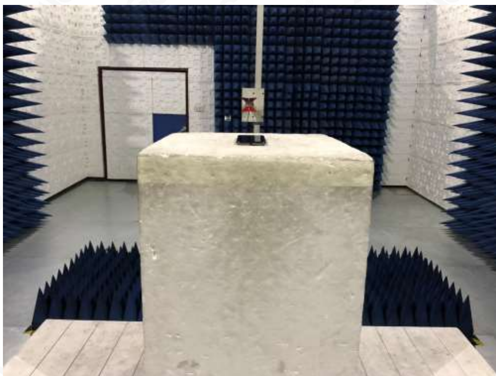
RADIATED SPURIOUS EMISSION-ABOVE 1G TEST SETUP
