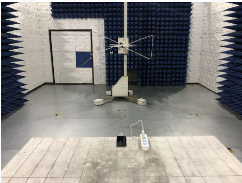
EN 55032 RADIATED EMISSION TEST SETUP
