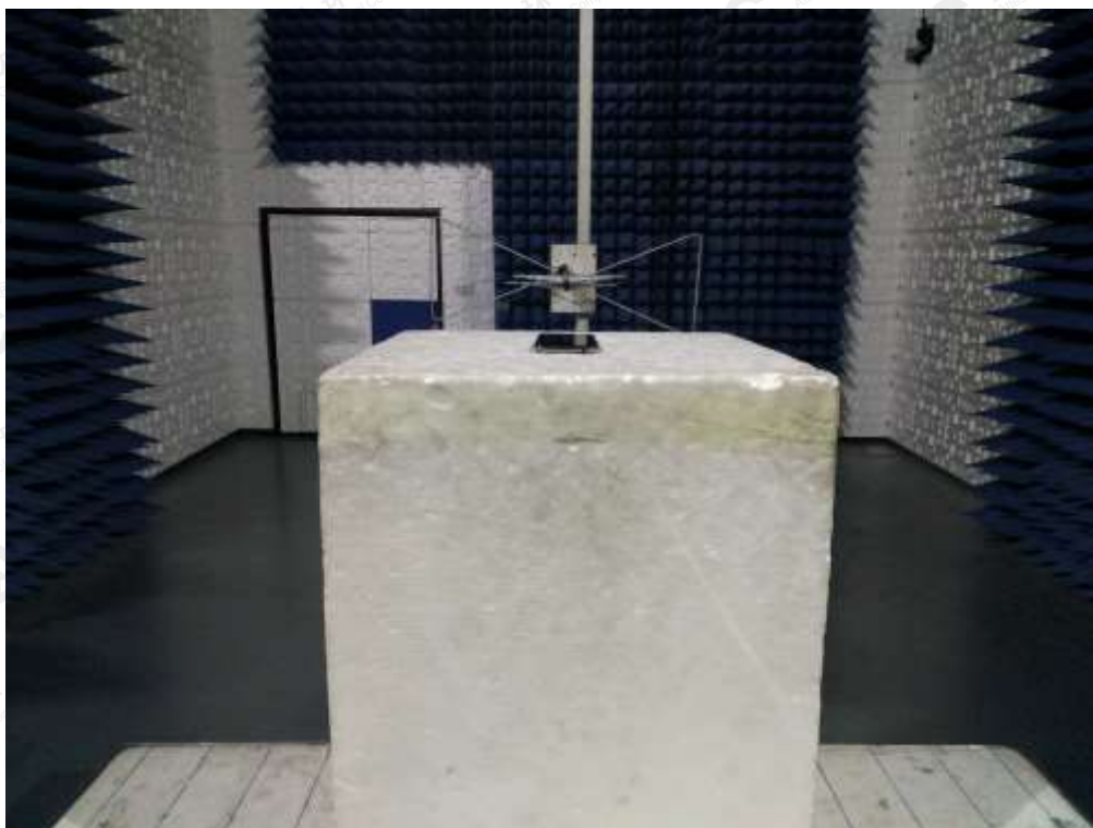
RADIATED SPURIOUS EMISSION-ABOVE 1G TEST SETUP
