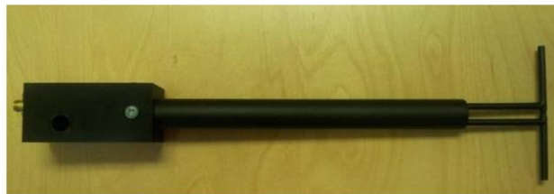
Figure 1 – MVG COMOSAR Validation Dipole
