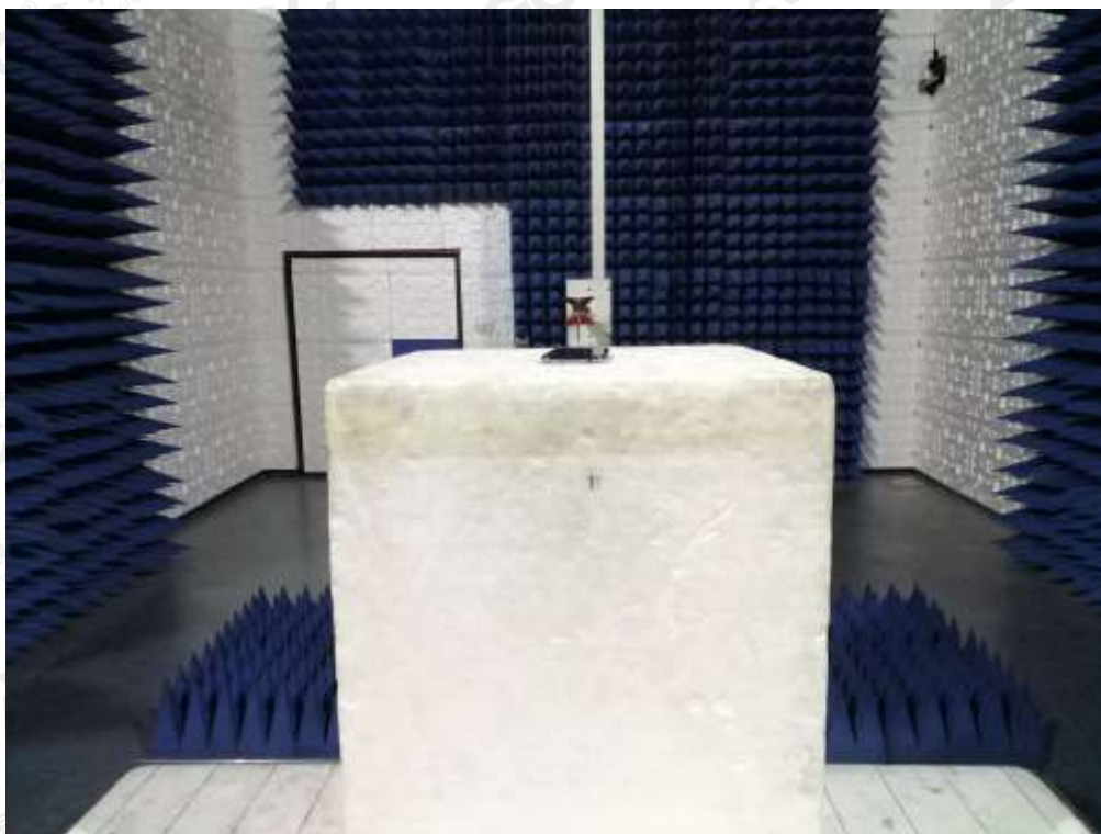
RADIATED SPURIOUS EMISSION-ABOVE 1G TEST SETUP
