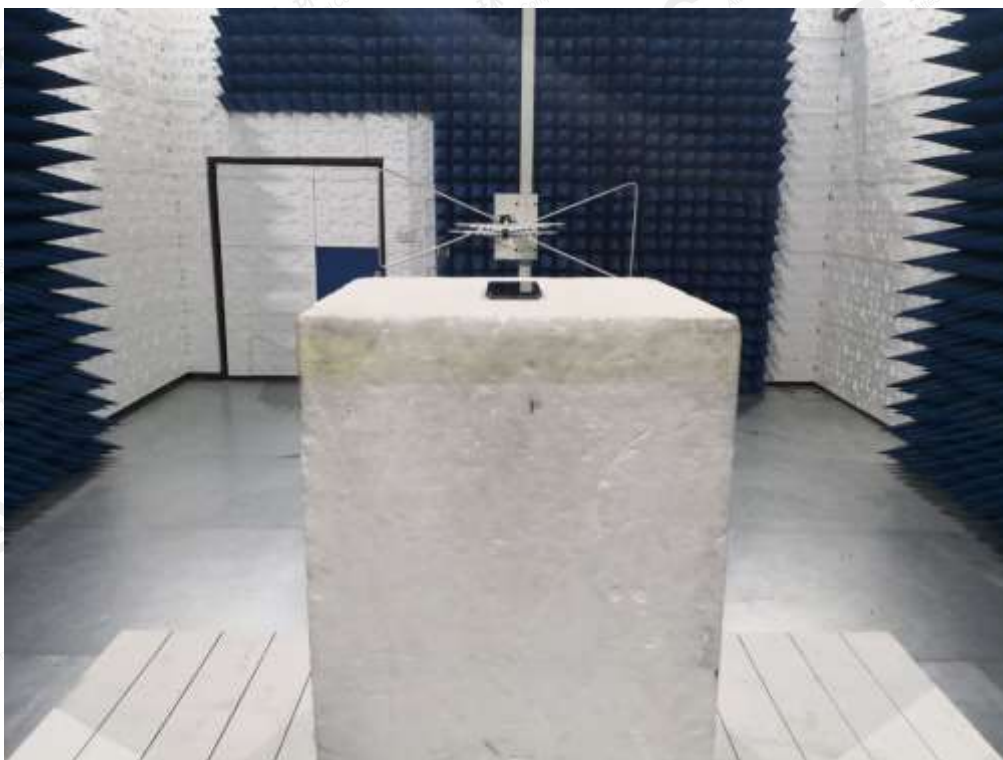
RADIATED SPURIOUS EMISSION-ABOVE 1G TEST SETUP
