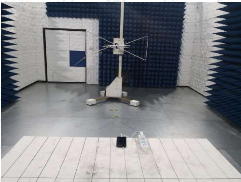
RADIATED EMISSION TEST SETUP
