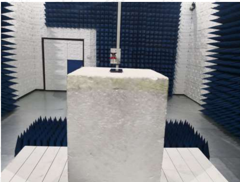
RADIATED SPURIOUS EMISSION-ABOVE 1G TEST SETUP
